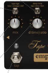
**tap stompswitch:** in tap mode, this sets the delay time when tapped. it will change to the new delay time after 2 taps and will average the last 4 taps
